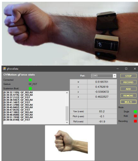
Figure 4. Example of a gesture with an EMG device attached and its processing in the application
