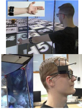
Figure 1. EMG device MYO (left), Optitrack devices (right) in LIRKIS laboratory during test
